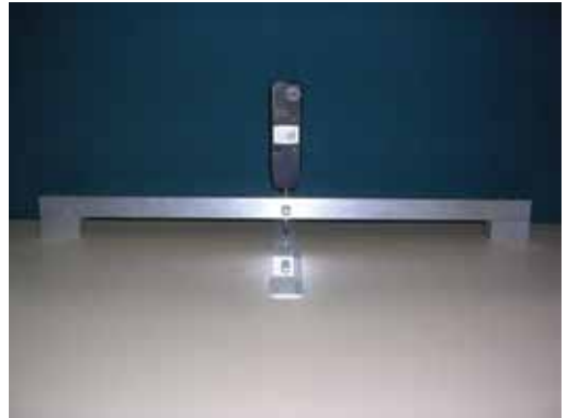
Digital gauge used to determine plasterboard joint compliance with AS 2589 'Gypsum linings – Application and finishing'
